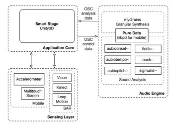
Fig 1. Smart Stage general architecture
